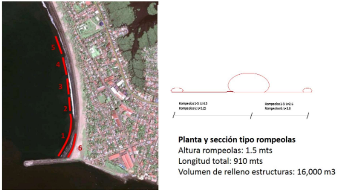
Figure 13 c-Geotubes location and technical data (Axisima, 2016)
